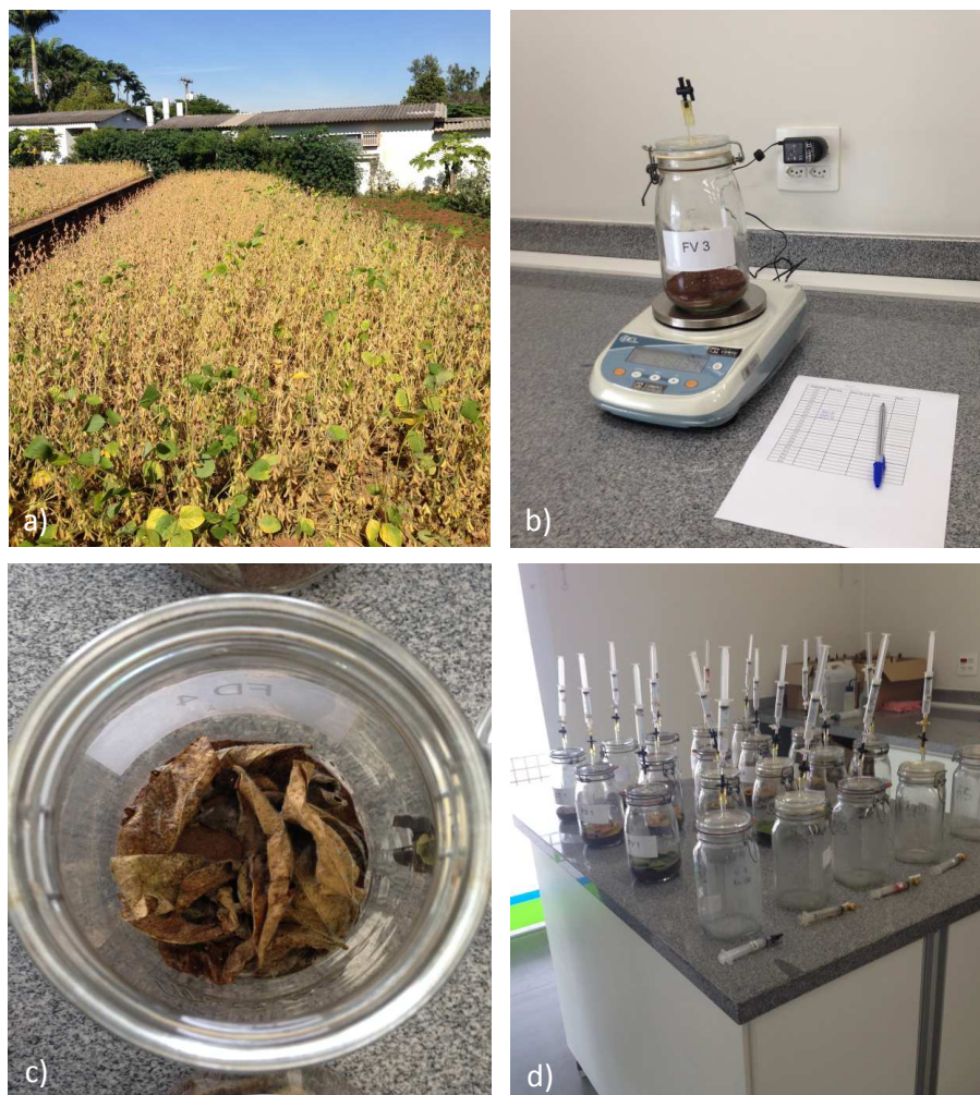
Figure 3.6 - a) Soybean cultivated in experimental plots; b) Daily weighting of jars for moisture control; c) Soybean plant material incubated in jars; d) Gas sampling for \text{N}_2\text{O} emissions.
