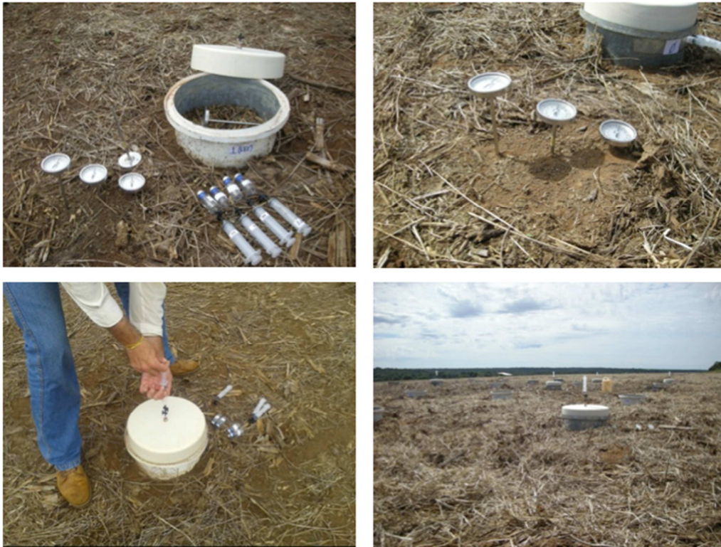
Figure 3.4 - Example of gas sampling procedures with static chamber in field conditions.
